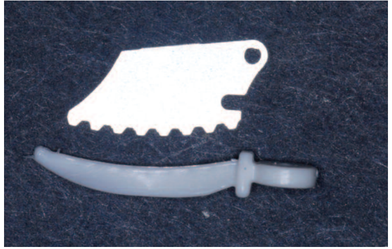
Figure 19b: Metal guard detached from the wedge.
