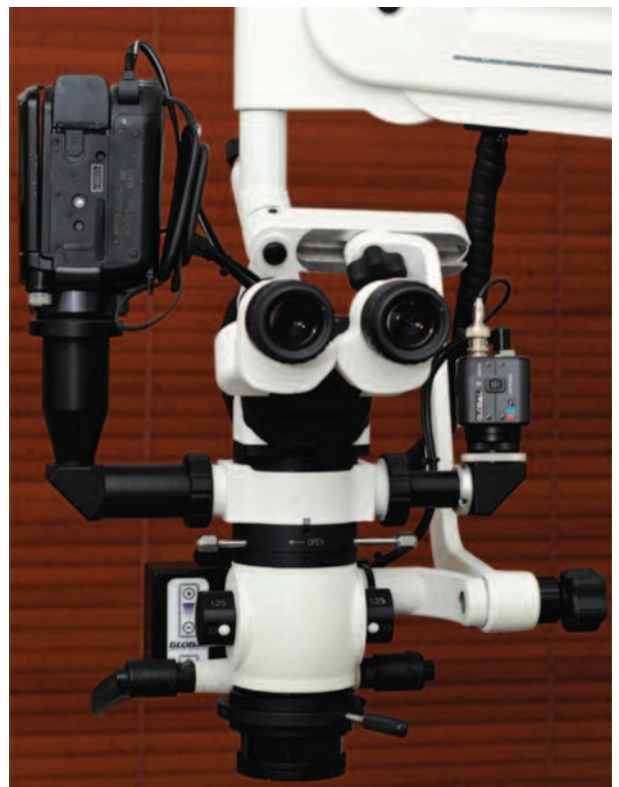
Figure 1: Global 6-Step Dental Operating Microscope (DOM) fitted with a dual-iris, LED light source, beam splitter and HD video camera.
