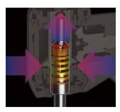
Unique, multi-point chuck MORITA's unique chuck design grips the bur firmly and doesn't lose its strength even after years of use. Experience the stability only a TORQTECH can provide when performing work that requires great precision.
